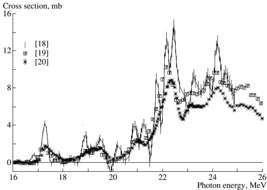
**Fig. 3.** Cross sections for the reaction  $^{16}\text{O}(\gamma, xn)$  according to data from an experiment with bremsstrahlung photons (the energy resolution there was 200 keV) [18] and from two experiments performed with quasimonoenergetic annihilation photons in Saclay [19] and in Livermore [20] (the resolution claimed in those studies was 180–280 and 200–300 keV, respectively).
