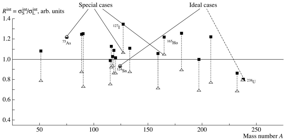
**Fig. 5.** The systematics [26] of values  $R^{\text{int}}(n) = \sigma_S^{\text{int}}(\gamma, n) / \sigma_L^{\text{int}}(\gamma, n)$  (■) and  $R^{\text{int}}(2n) = \sigma_S^{\text{int}}(\gamma, 2n) / \sigma_L^{\text{int}}(\gamma, 2n)$  (Δ). Special cases— $(\gamma, 2n)$  cross section ratios are more than 1.0. Ideal cases— $(\gamma, n)$  and  $(\gamma, 2n)$  cross section ratios are near. Special cases and ideal cases were processed individually [26].
