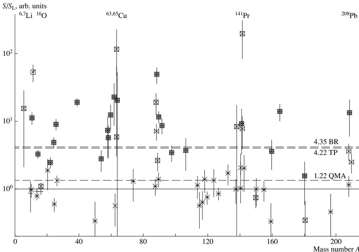
**Fig. 2.** The systematics of ratios  $S/S_L$  (see text) obtained for the total photoneutron reaction cross section data: BR data [( $\boxtimes$ ) Moscow, ( $\boxplus$ ) Melbourne (Australia), ( $\boxminus$ ) other]; QMA data [( $\ast$ ) Saclay (France), ( $+$ ) Giessen (Germany), ( $\times$ ) other]; TP data [( $\boxtimes$ ) Illinois (USA)].
